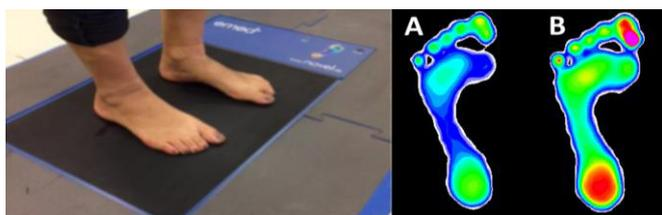
**Figure 1:** Hallux and toes strength test using an emed pressure platform (A-Baseline, B- after 12 weeks of intervention).
