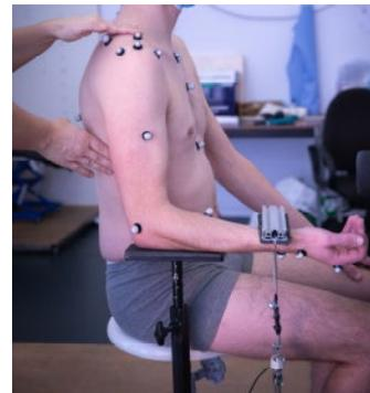
Figure 1: Elbow isometric MVC measurement device.
