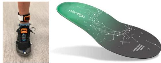
**Figure 1:** Tibia-mounted (IMeasureU), lace-mounted (RunScribe), and insole-embedded (Plantiga) inertial measurement units.
