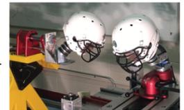
Videos used to guide laboratory reconstructions with mounted accelerometers
